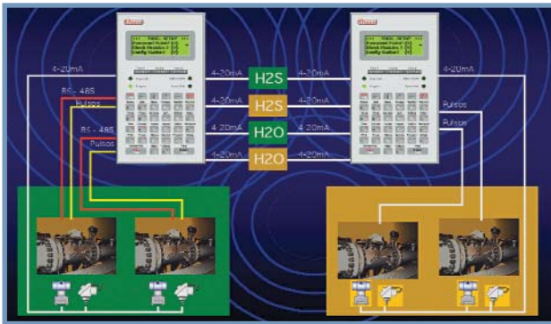
Redundant ultrasonic meters, gas chromatographs; H 2 O and H 2 S.
