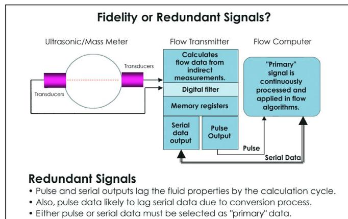
Figure 3. The combining of the two signal types – pulse and serial – cannot achieve meaningful fidelity checks, only signal redundancy.
