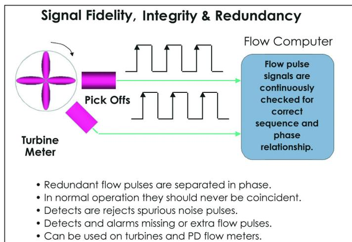
Figure 2. Pulse signals are checked for discrepancies; alarms are reported where discrepancies exceed a specific threshold.
