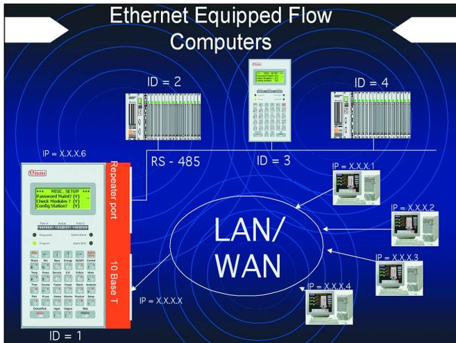
Figure 4. Each flow computer is connected serially to the same redundant ultrasonic meters, redundant gas chromatographs, local PCs and redundant H<sub>2</sub>O and H<sub>2</sub>S analyzers.
