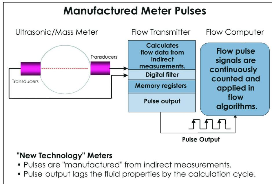
Figure 1. New technology meters are based on a calculation and measurement cycle time, during which a series of indirect measurements are taken, several calculations made and the results stored in memory.
